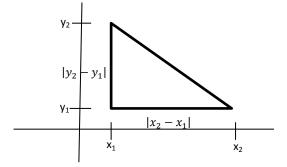
The lengths of the legs are  $|x_2 - x_1|$  and  $|y_2 - y_1|$ . The distance between the points  $(x_1, y_1)$  and  $(x_2, y_2)$  is the hypotenuse of the triangle. Applying the Pythagorean Theorem,  $d^2 = (x_2 - x_1)^2 - (y_2 - y_1)^2$ . Since distance is non-negative, then the distance, d, between the points is given by
